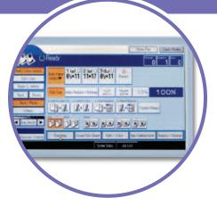
The large, full-color W-VGA control panel makes it easy to program jobs in seconds. It also offers a Simplified Display option and animated user guidance for common tasks.
